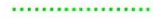
804 Track, slow 0.8-1 m Colour: upper green (PMS 354) Diameter of dots 0.7 mm and distance between dots 1.3 mm
